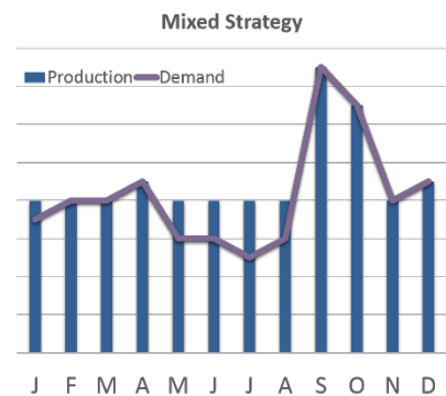
Figure 28. In this mixed strategy, the production increases with demand, but never drops below a certain value when demand is low. Developed by LINC in Supply Chain Management Consortium.
