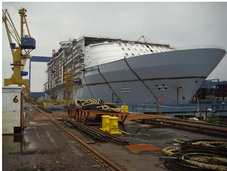
Figure 16. Large sea-faring vessels such as this one are too large to move around during construction. Hence, the workers and supplies come to it. By ComradeWolf at en.wikipedia.org [Public domain], via Wikimedia Commons.
