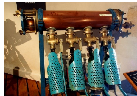
Figure 59. Even older models had a mechanical shut off valve that would prevent the bottles from overfilling if the regular valve failed. By AlfvanBeem (Own work) [CC0], via Wikimedia Commons.
