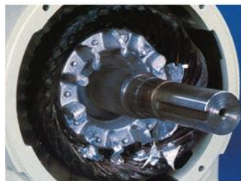
Locked rotor overload damage to all windings (may also be caused by excessive starts or reversals)
