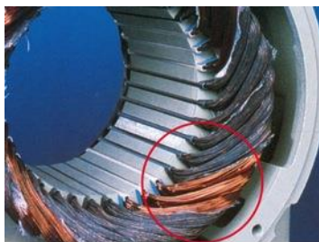
Single-phased undamaged winding (caused by a missing voltage phase in a wye-connected motor)
