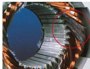
Single-phased damaged winding (caused by a missing voltage phase in a delta-connected motor)
