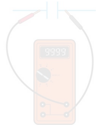
INFINITE RESISTANCE = OPEN CONTACTS
