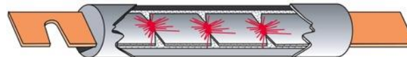
When subjected to a short circuit, several sections of the fuse link melt almost instantly.
