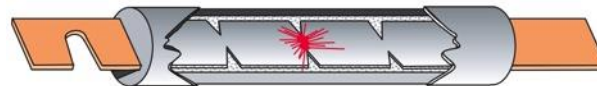
Under sustained overload, a section of the link melts and an arc is established.
