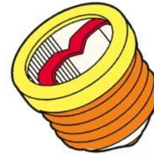
EDISON-BASE FUSE (MAXIMUM RATING 30 AMPERES)
