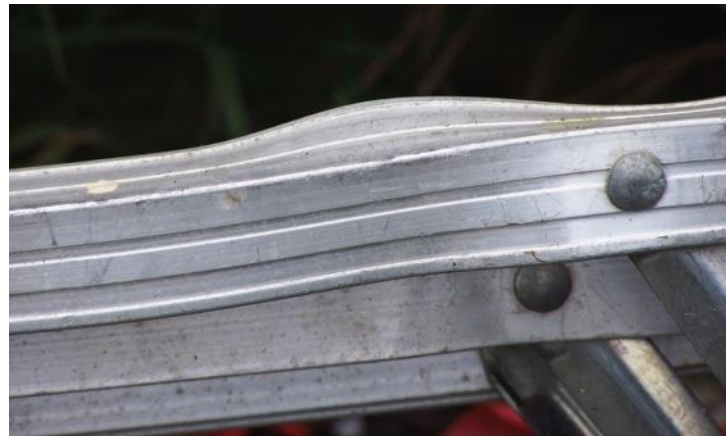
(C) BENT BACK BRACE
