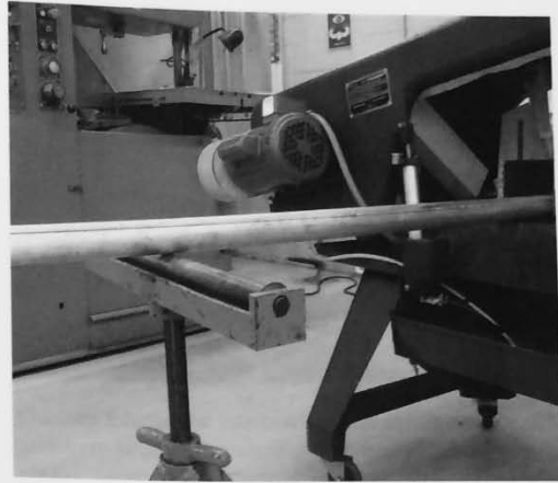
FIGURE 3.4.5 Use a stand to support long bars being cut on the horizontal band saw. This keeps them flat and prevents them from falling when the vise is unclamped.
