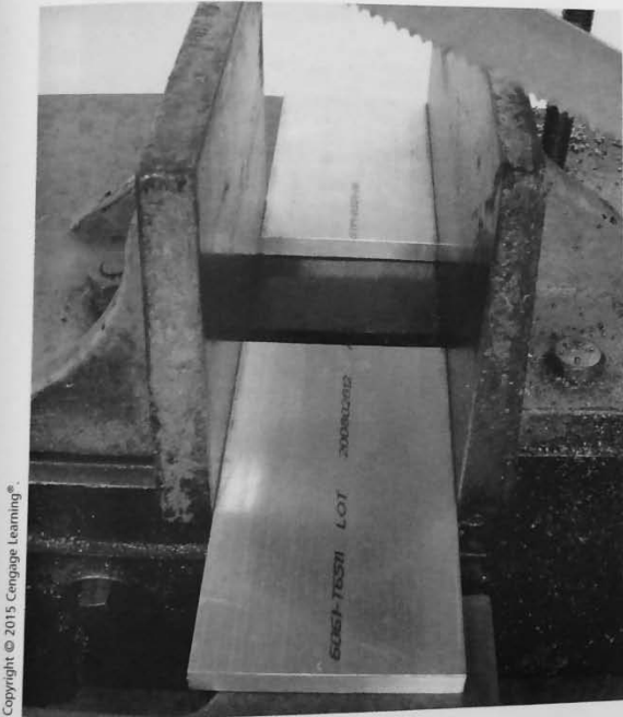
FIGURE 3.4.4 When clamping short sections in the saw vise, use another piece of the same size material to keep the moveable jaw parallel to the solid jaw to ensure adequate clamping.
