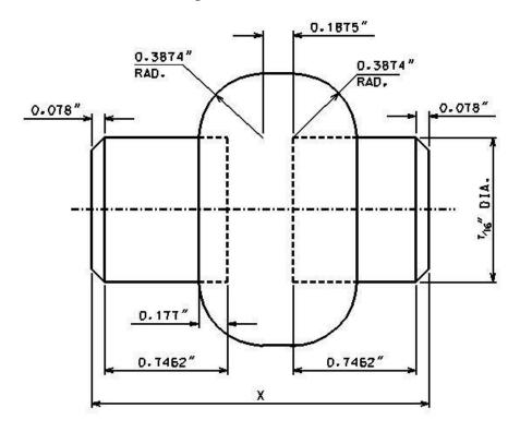
2. Find the total length X of the buttonhead assembled rivet shown.
