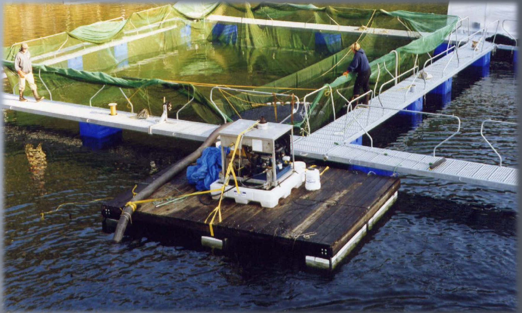
Transporting fish from freshwater net pen to saltwater using a fish pump
