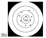
The above image is an example of a. good accuracy, good precision \*b. good accuracy, bad precision c. bad accuracy, good precision d. bad accuracy, bad precision
