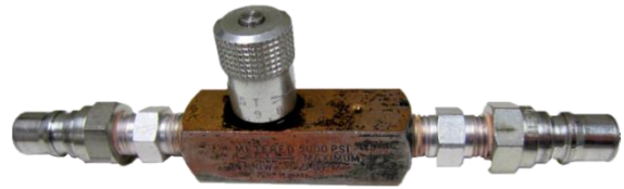
Flow Control Valve
