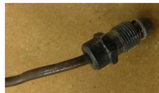
The part of the thermocouple that connects to the gas valve
