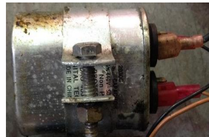
Fan Motor Run Capacitor on Conveyor Oven
