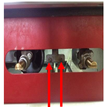
Pilot Light valves
