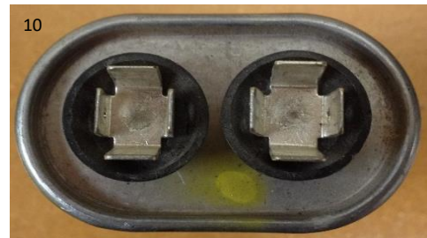
Top Terminals of a run capacitor
