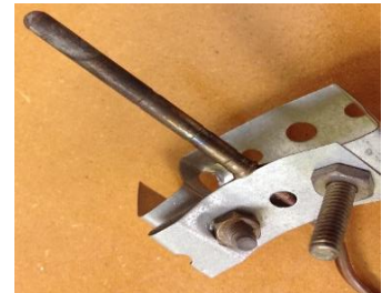
The part of the thermocouple that sits in the flame
