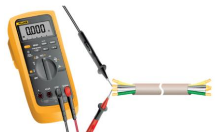
Testing Continuity of a Wire
