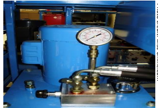
Hydraulic Power Unit
