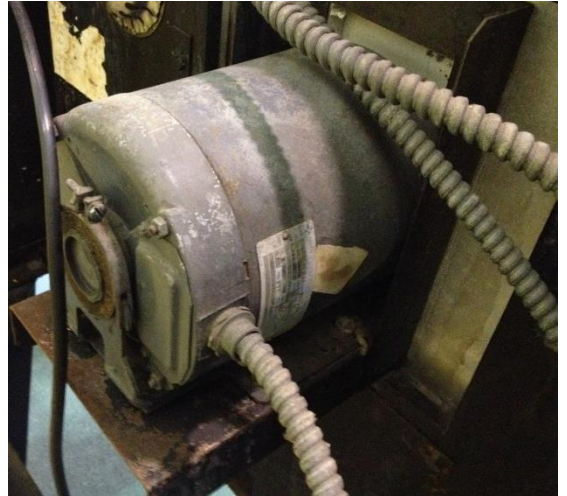
Fan Motor on Convection Oven
