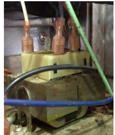
Transformer in a conveyor oven
