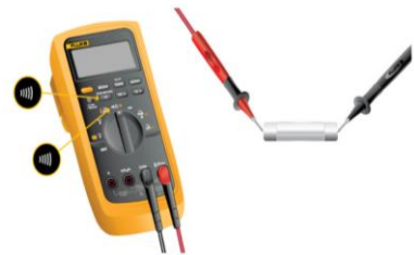
Testing Continuity of a Fuse
