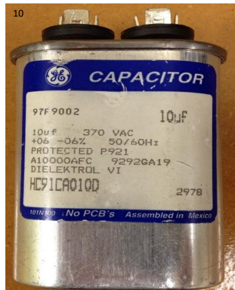
10 microfarad run capacitor
