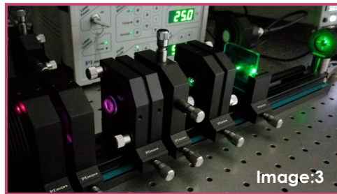
Nd:YAG laser setup, alignment, and characterization with Frequency Doubler
