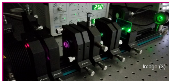
Nd:YAG laser setup, alignment, and characterization with Frequency Doubler
