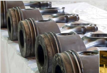
Piston rings sealing properly. Showing a good ring seal and no compression entering crankcase area
