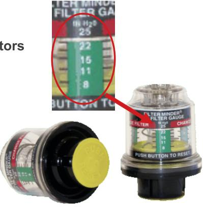
Air cleaner monitors are designed to also measure inches of H20 air inlet restrictions. They are located in the same location a technician would make the measurement using a slack to monometer or gauge.
