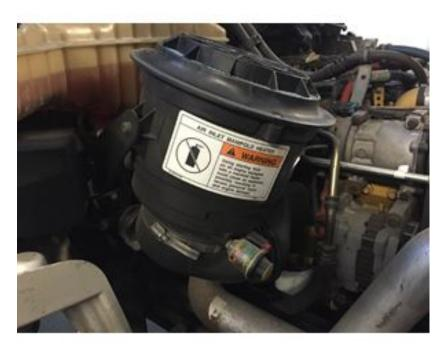
Almost all diesel engines have the same air restriction specifications; Clean filter 10 inches of H2O Dirty filter maximum 20 inches of H20
