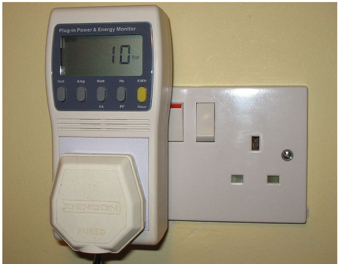
Figure 12–6: A plug-in power meter measures the amount of power being drawn by the connected appliance. (Source: Gareth.randall/Creative Commons (Public Domain)/ https://commons.wikimedia.org/wiki/File:Plug-in_Power_%26_Energy_Monitor_in_UK_Domestic_Mains_Socket.jpeg )
