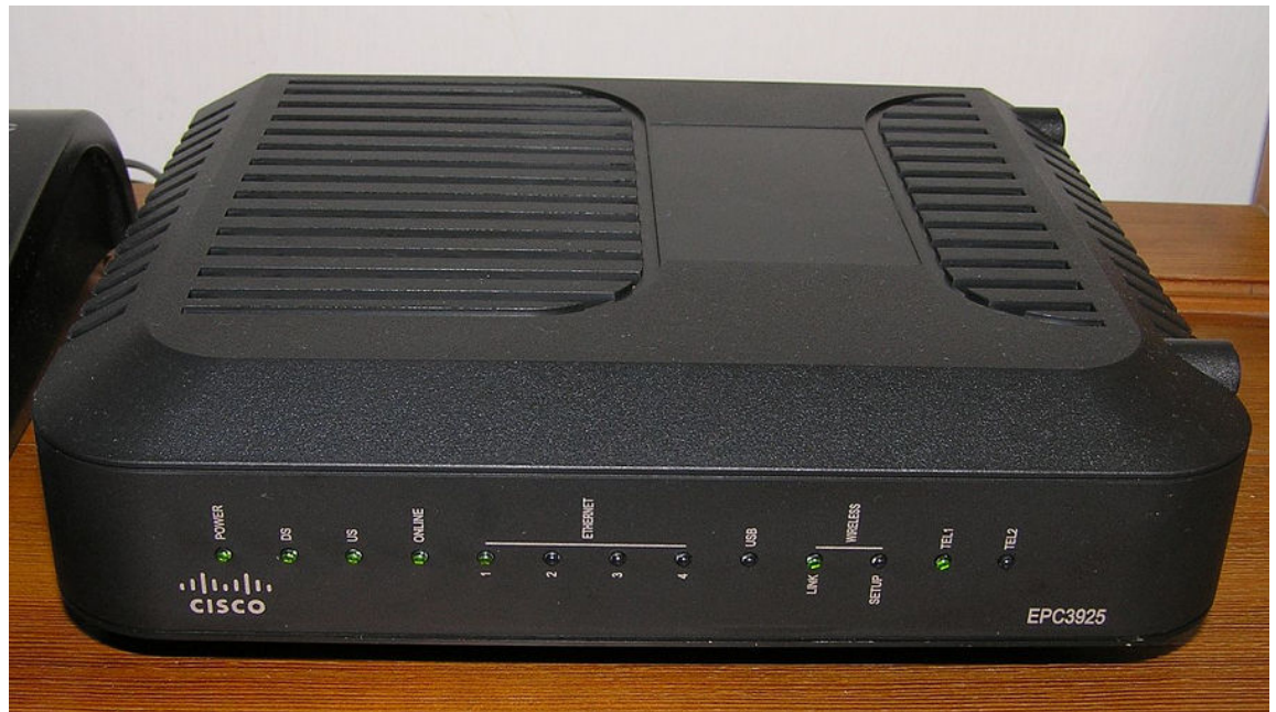
Figure 10–5: A cable modem acts as a gateway for a residential network. (Source: Larocomp/ Creative Commons (Public Domain)/ https://commons.wikimedia.org/wiki/File:EPC3925.jpg )
