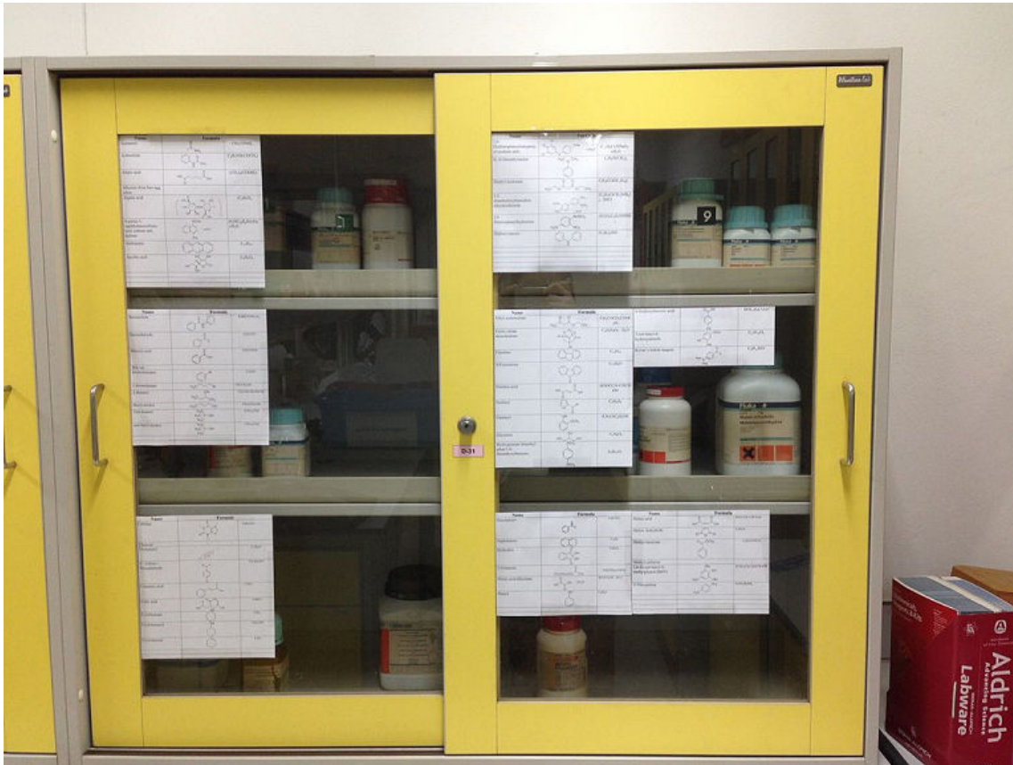
Figure 7-5: Chemicals stored securely in a chemical cabinet. (Source: U5680336/Creative Commons (CC BY-SA 4.0)/ https://commons.wikimedia.org/wiki/File:Chemical_cabinet3.JPG )
