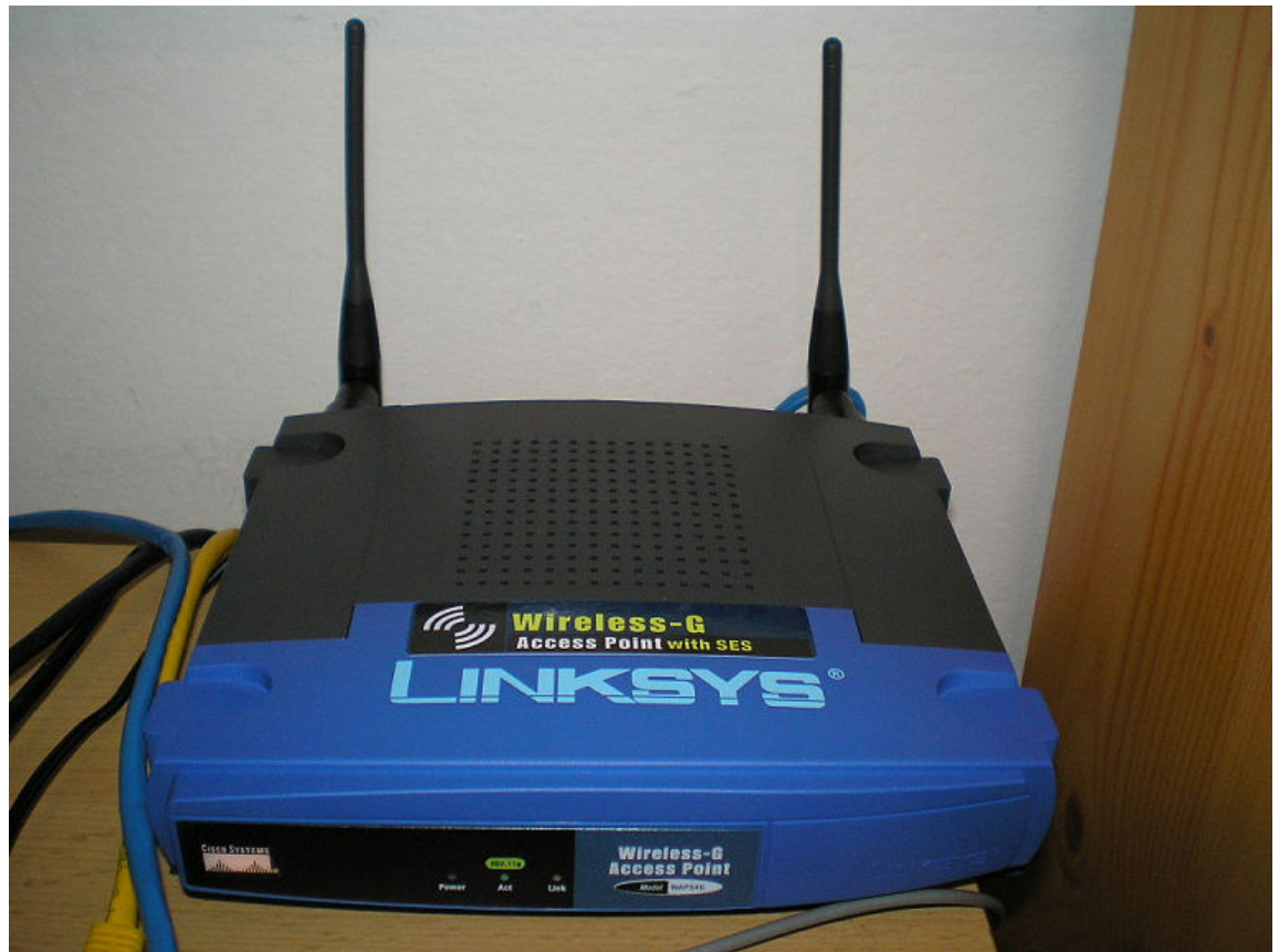
Figure 11-6: A wireless access point creates a Wi-Fi network from a wired connection. (Source: Macic7/Creative Commons (CC BY-SA 3.0)/ https://commons.wikimedia.org/wiki/File:Linksys_WAP54G.JPG )
