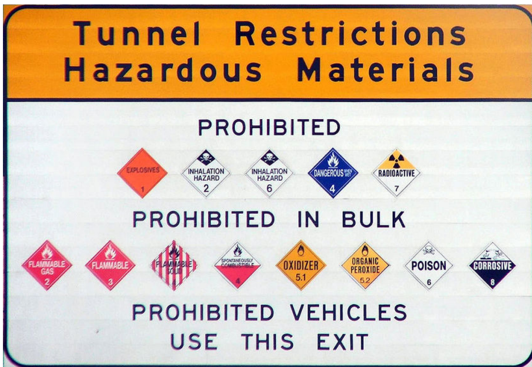
Figure 7-10: A sign on the Pennsylvania Turnpike denotes which hazardous materials are prohibited from being transported through a tunnel along the highway. (Source: Shanel/Creative Commons (Public Domain)/ https://commons.wikimedia.org/wiki/File:Prohibitionboard.jpg )
