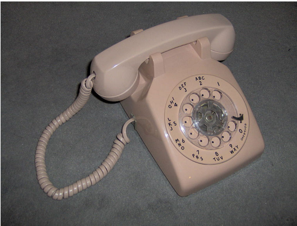
Figure 11-1: A rotary phone operated using the Plain Old Telephone System transmission protocol. (Source: ProhibitOnions/Creative Commons (Public Domain)/ https://commons.wikimedia.org/wiki/File:WE500dialphone.jpg )
