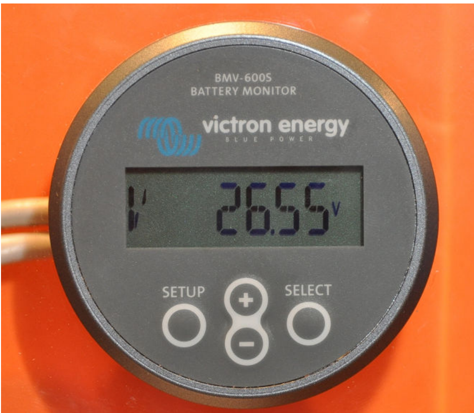
Figure 12-2: A battery monitor. (Source: S.J. de Waard/Creative Commons (CC BY-SA 3.0)/ https://commons.wikimedia.org/wiki/File:Amsterdam_RAI_METS_2011_(138).JPG )
