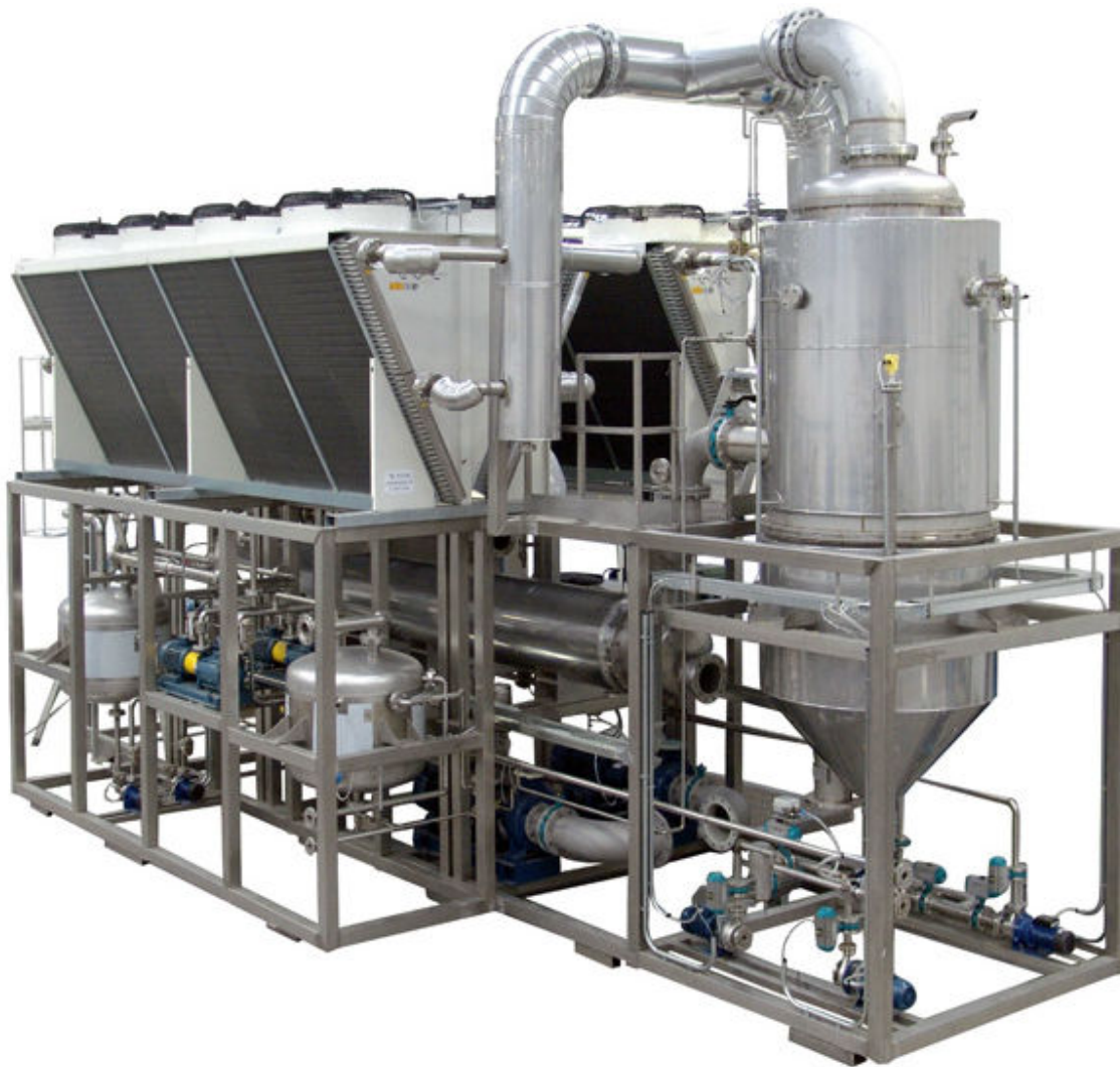
Figure 5-4: A vacuum evaporator. (Source: Condorchem/Creative Commons (CC BY-SA 3.0)/ https://commons.wikimedia.org/wiki/File:Vacuum_evaporation_plant.jpg )
