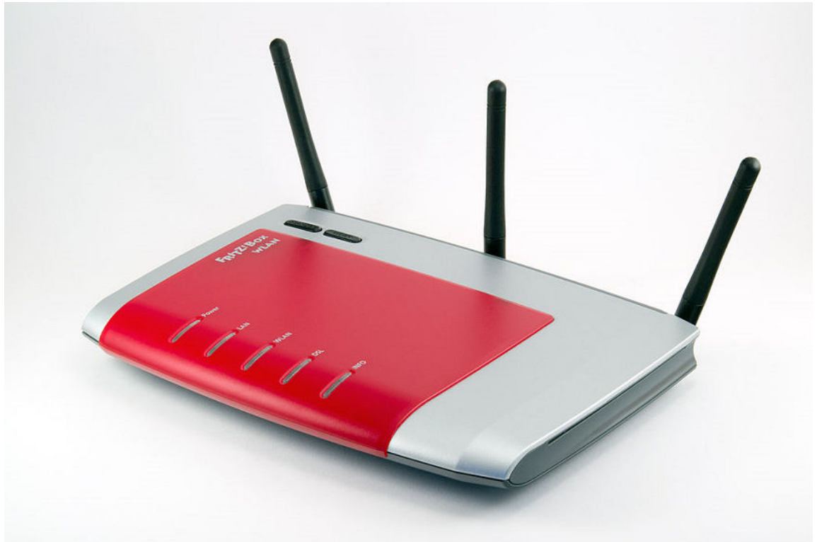
Figure 10–3: A wireless router. (Source: Tors/Creative Commons (Public Domain)/ https://commons.wikimedia.org/wiki/File:AVM_FRITZ!Box_WLAN_3270.jpg )
