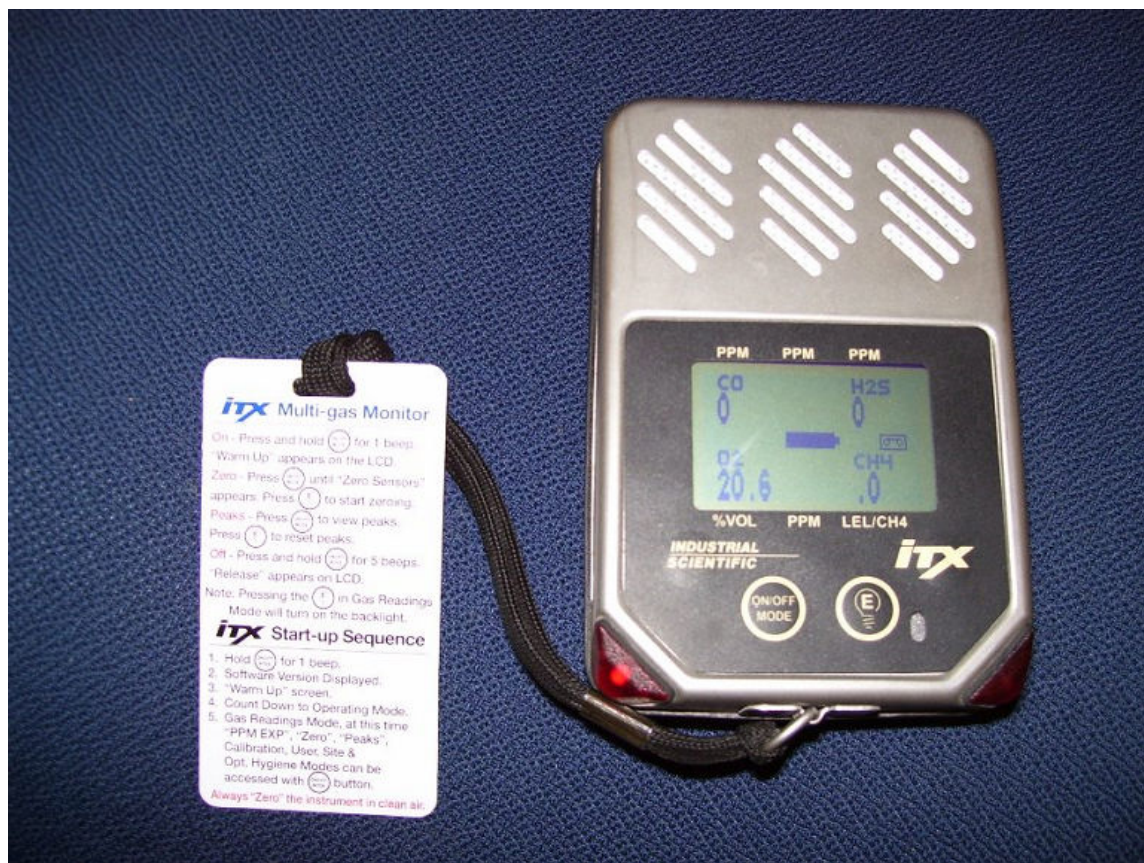
Figure 7-9: A portable gas detector can be used to monitor hydrogen concentration. (Source: Sansumaria/Creative Commons (CC BY-SA 3.0)/ https://commons.wikimedia.org/wiki/File:Detector_for_Gas.jpg )
