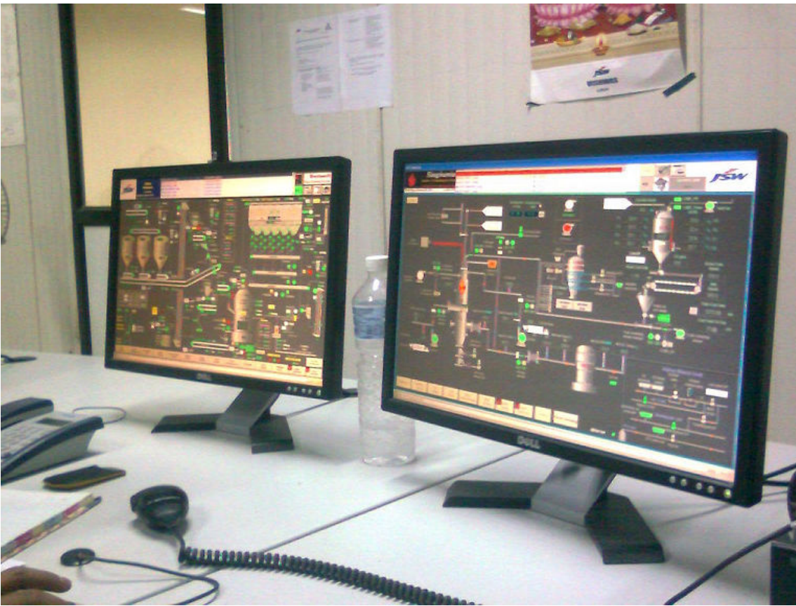
Figure 12–9: A SCADA system displays information for the various connected components. (Source: Sunilshamnur/Creative Commons (CC BY 3.0)/ https://commons.wikimedia.org/wiki/File:Chemengg.jpg )
