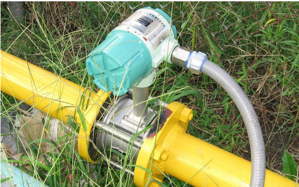
Figure 12-1: A flowmeter. (Source: Cmarcante/Creative Commons (Public Domain)/ https://commons.wikimedia.org/wiki/File:VORTEX_Montado_v1.JPG )
