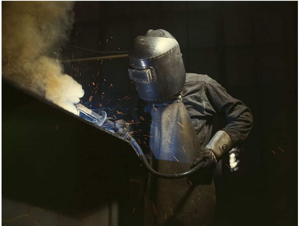
Figure 13–5: Welding work within the MCO facility requires a hot work permit. (Source: Library of Congress/Creative Commons (Public Domain)/ https://commons.wikimedia.org/wiki/File:AlfredPalmerwelder1.jpg )
