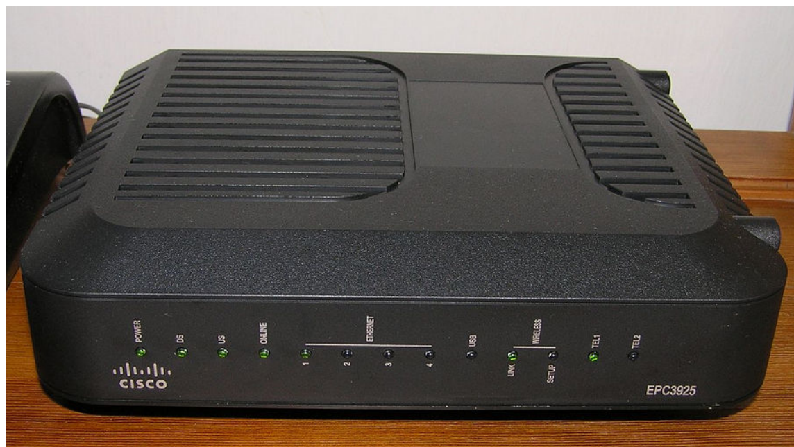
Figure 10–5: A cable modem acts as a gateway for a residential network. (Source: Larocomp/ Creative Commons (Public Domain)/ https://commons.wikimedia.org/wiki/File:EPC3925.jpg )
