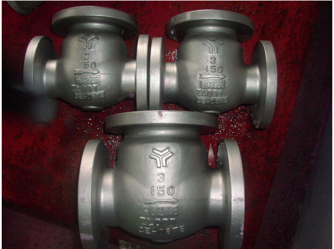
Figure 5-3: Check-valves keep the flow of the plumbing system moving in one direction. The arrows on these check valves show the direction that fluid is moving. (Source: The Alloy Valve Stockist (Heather Smith)/Creative Commons (CC BY 3.0)/ https://commons.wikimedia.org/wiki/File:Swing_Check_valves.JPG )
