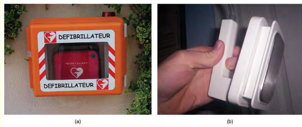
Figure 19.26 Defibrillators (a) An external automatic defibrillator can be used by nonmedical personnel to reestablish a normal sinus rhythm in a person with fibrillation. (b) Defibrillator paddles are more commonly used in hospital settings. (credit b: “widerider107”/flickr.com)
