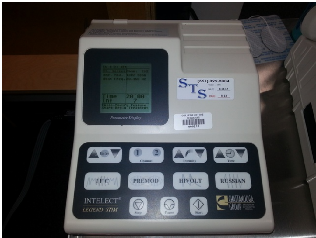
EStim Machine This is the interface of an EStim machine that will provide the electrical current to the patient's muscles.
